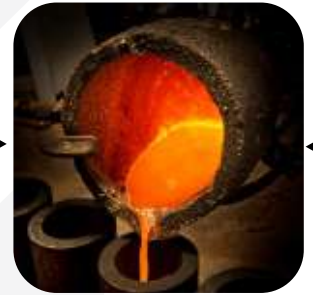
Addition of Ferror Alloys & other elements
