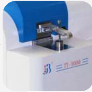
Testing of liquid metal by spectro metre
