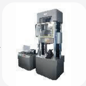
TMT testing by UTM Machine
